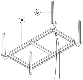
ATTACH LEG (B) TO THE TOP TABLE (A) BY ALIGNING INTO WOODEN CORNER HOLES, AND SECURED BY HEXAGONAL BOLTS (BB). TIGHTEN BY USING WRENCH (AA).
